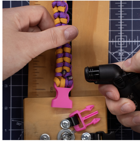
25. Use a lighter to melt the freshly trimmed EBNPS end for 3 to 6 seconds.
